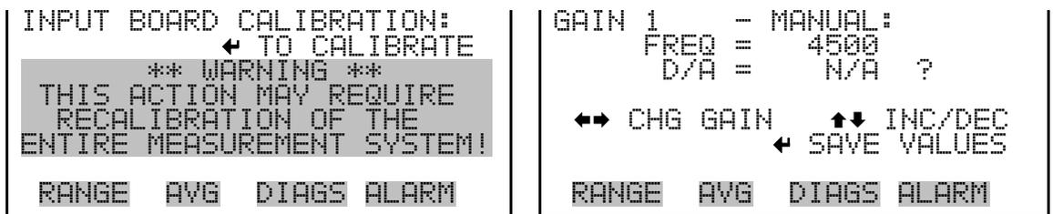
**Automatic Input Calibration** The Automatic Input Calibration screen is used to do an automatic calibration of the input board A/D stages. A message will be displayed after the optimum setting has been determined.
